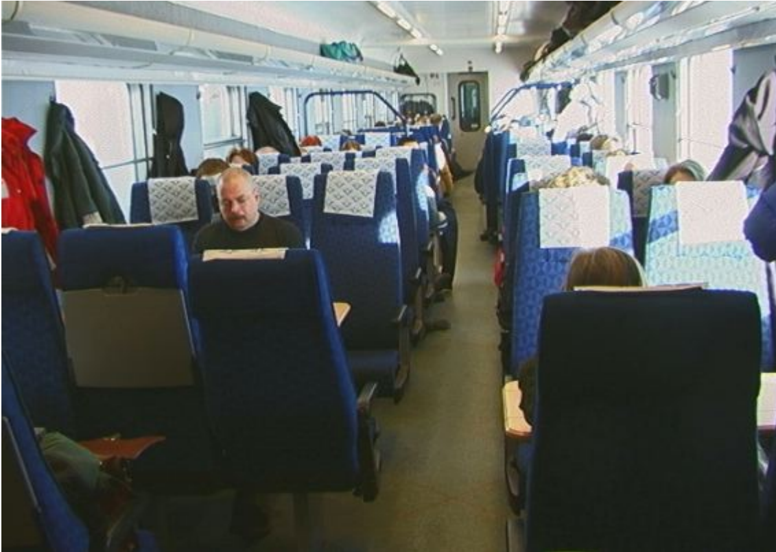
Figure 6. Interior of the "InterRegioMax" test coach with 2 + 3 seating. Photo: Kottenhoff)
